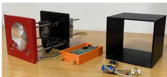
Figure 3: Components of new hardware version, extensive use of 3d-printed components, off-the-shelf electronics, and open-source hardware designs minimize costs.
