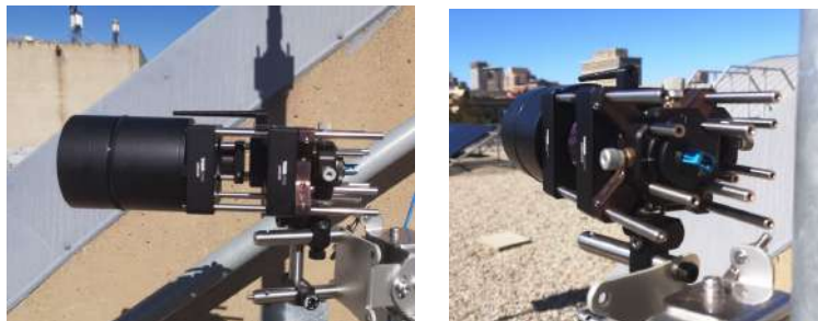
Figure 1: Bidirectional FSO system which couples light between two fibre optic cables
